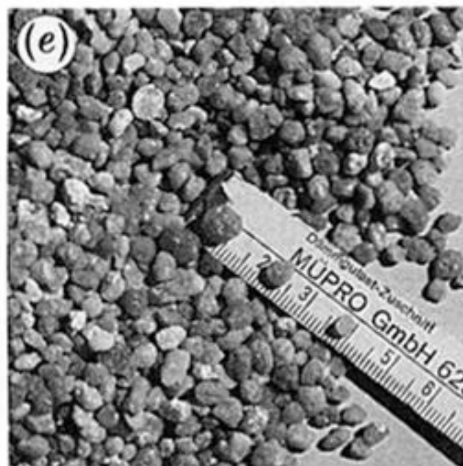
Figure 7. Samples of the granular materials: (a) glass 0 (3 mm); (b) glass 1 (5 mm); (c) Vestolen; (d) quartz 0 (3 mm); (e) quartz 1 (5 mm); (f) marmor 0 (3 mm); (g) marmor 1 (5 mm).
